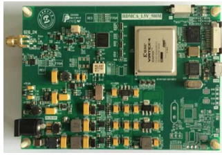
图 7 单板 500 MHz 数字化多道实物图 Fig.7 Physical picture of single board 500-MHz digital multi-channel.
